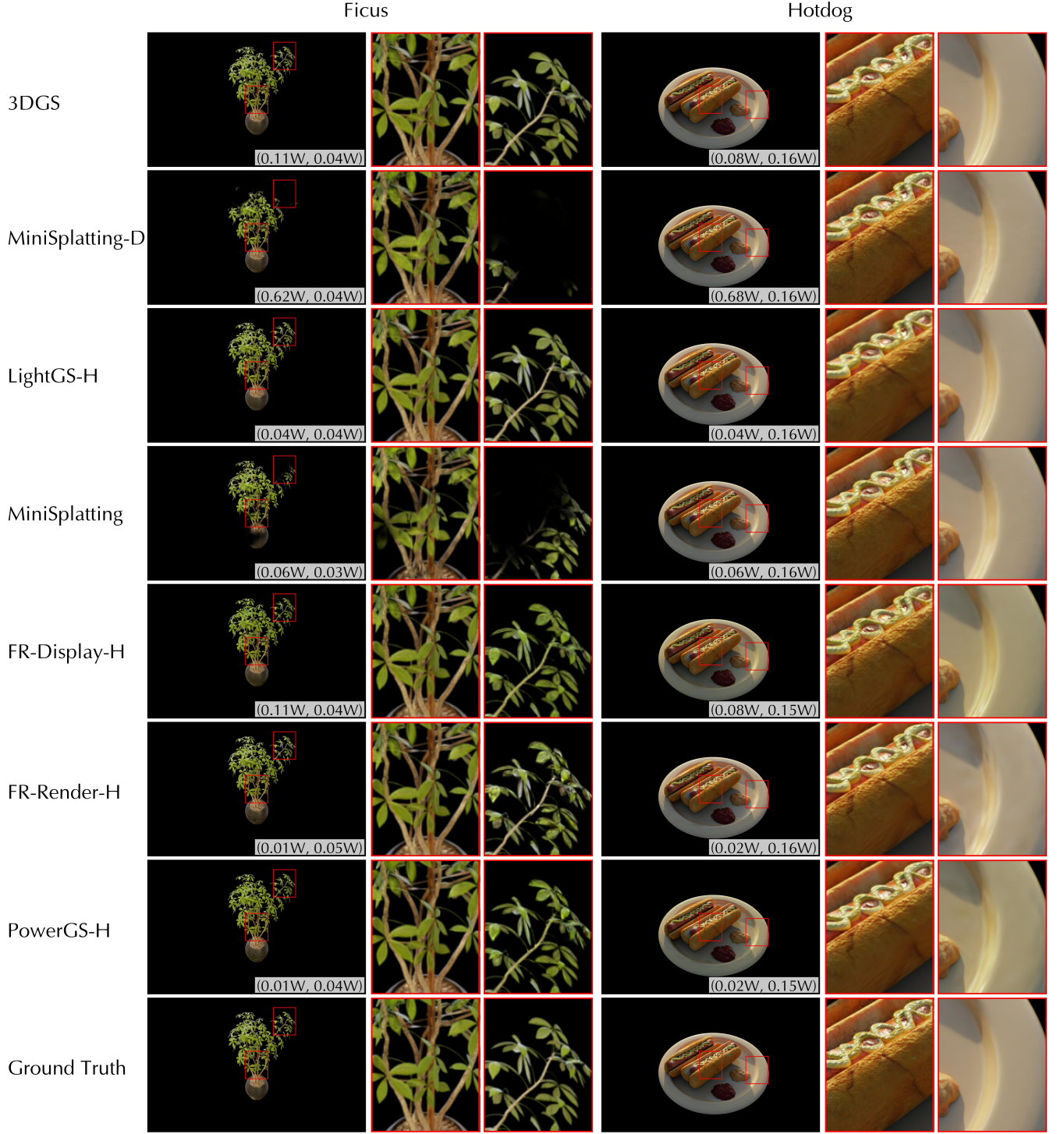
Fig. 10. Qualitative Evaluation. Rendered images of two scenes in Synthetic NeRF are shown, with annotated values for (rendering power, display power). Zoom-in views of the fovea region (left) and the periphery (right) are also provided. For all foveated versions, the gaze is fixed at the center of the image.
