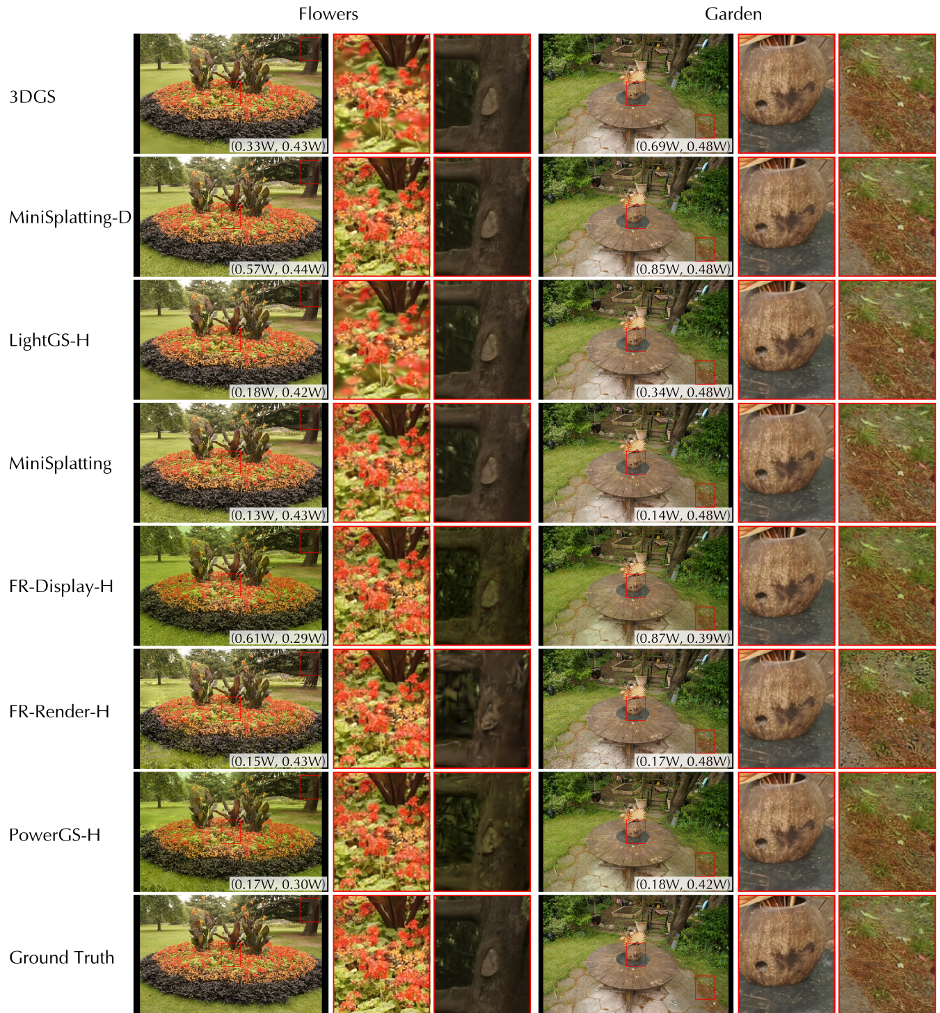
Fig. 4. Qualitative Evaluation. Rendered images of two scenes in Mip-NeRF360 are shown, with annotated values for (rendering power, display power). Zoom-in views of the fovea region (left) and the periphery (right) are also provided. For all foveated versions, the gaze is fixed at the center of the image.
