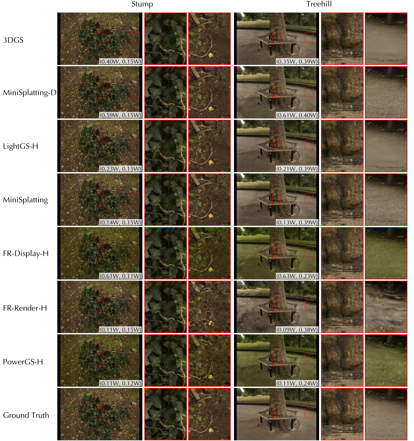
Fig. 6. Qualitative Evaluation. Rendered images of two scenes in Mip-NeRF360 are shown, with annotated values for (rendering power, display power). Zoom-in views of the fovea region (left) and the periphery (right) are also provided. For all foveated versions, the gaze is fixed at the center of the image.
