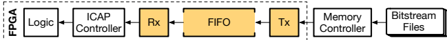
Fig. 9: Runtime partial reconfiguration engine. Augmentations to existing hardware on the Zynq board are shaded.
