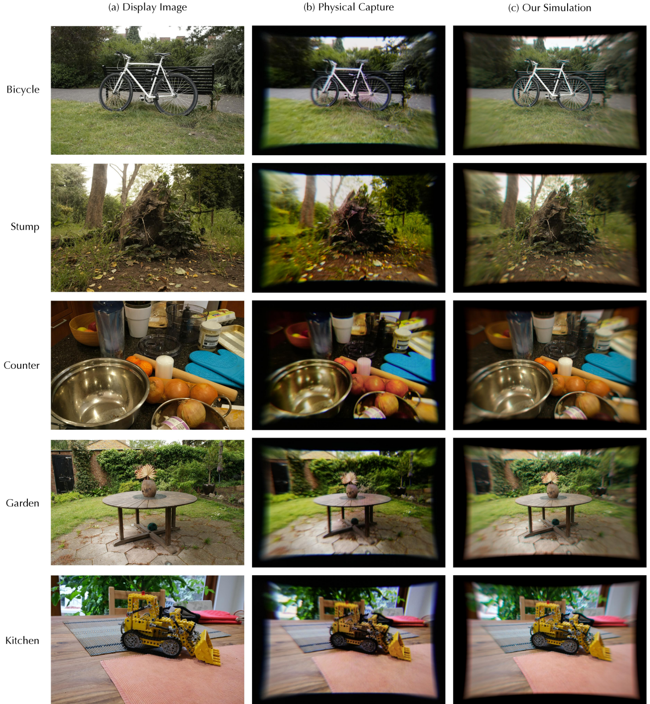
Fig. S3. Camera-based verification of the display-optics simulation against real captures. We display the input image on an AMOLED display and capture the result through a Google Cardboard lens using a calibrated Sony FE 24–70mm F2.8 GM II camera. Left: input image shown on the display. Middle: calibrated camera capture through the real lens. Right: simulated result from our display-optics model. Remaining color differences may come from the simplified emission spectrum model of the display, camera sensor response functions, and potential Image Signal Processor (ISP) post-processing, which are not fully accounted for in our simulation.
